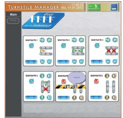
TMON SOFTWARE - software application for easy remote control of the turnstiles and gates
